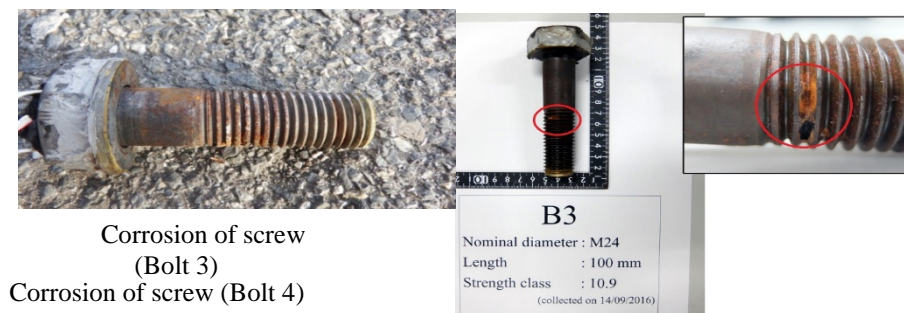
Figure 6: Corrosion of high strength bolts
