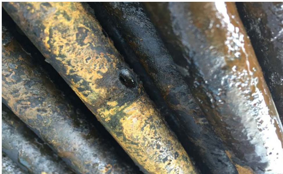
Figure 1b: Pitting Corrosion (Erbil refinery, Heat Exchanger)
