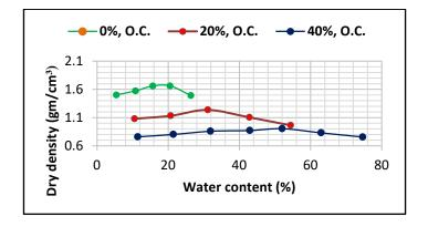
Figure 9: Compaction curves for different organic contents
