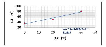
Figure 6: Liquid limit versus organic content
