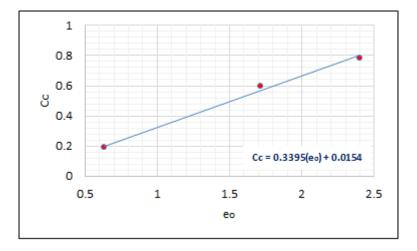
Figure 14: Variation of compression index with void ratio
