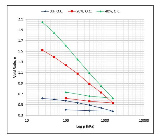
Figure 12: Void ratio versus logarithm of consolidation pressure for different percentages of organic soils.
