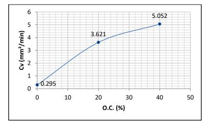
Figure 15: Effect of organic content on coefficient of consolidation
