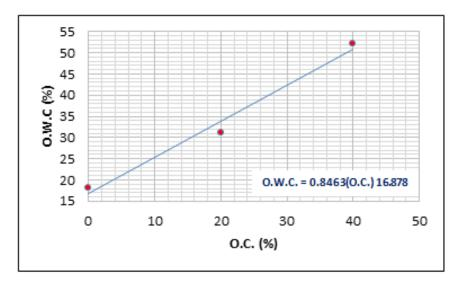
Figure 11: Optimum water content versus organic content
