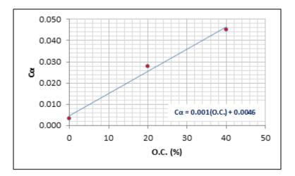
Figure 16: Effect of organic content on coefficient of secondary compression
