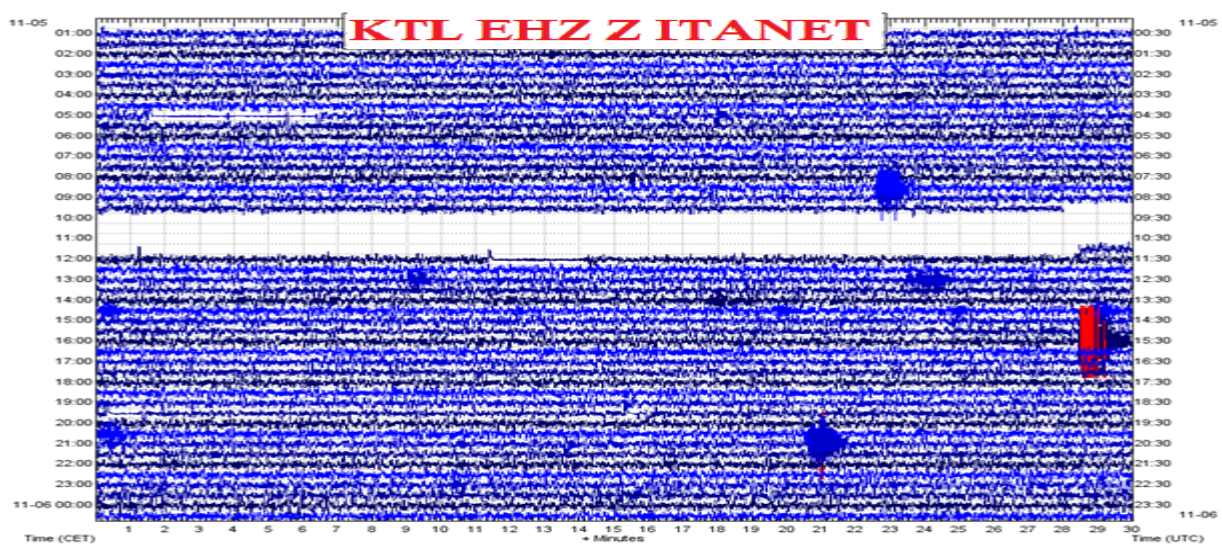
Figure 2: Helicorder of on day plot of the KTL records on 06/11/2011, the day of Nyamulagira eruption. In the records many volcanic tremors with detected hybrid events.
