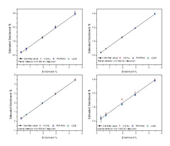
**Figure 2:** Calculated enrichment using MGAU, PC/FRAM and MGA codes using different detectors with different resolutions.
