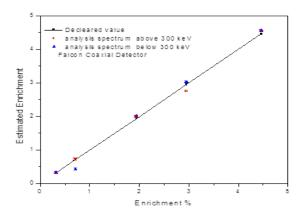
Figure 4: Obtained enrichment using MGAU and two energy segment spectral analysis
