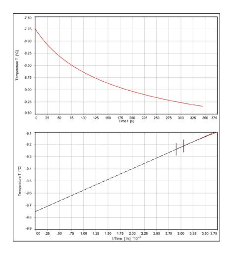
Figure 9: Express Temperature Measurement in TCPT-01 at the depth of 0.28 m
