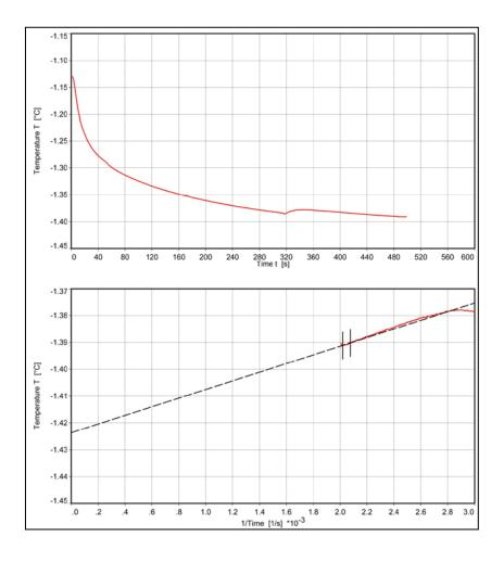
Figure 10: Temperature Measurement in TCPT-01 at depth of 5.38 m according to STO 36554501-049-2016 requirements
