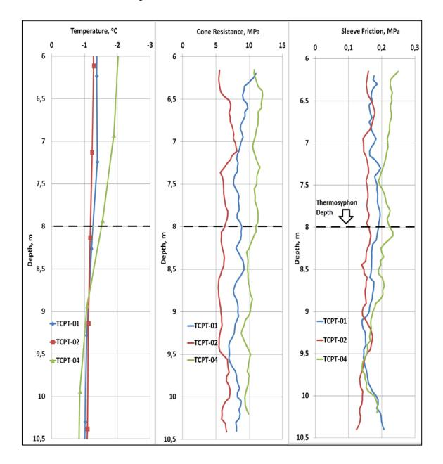
Figure 15: Temperature, Cone Resistance q<sub>c</sub> and Sleeve Friction f<sub>s</sub> vs Depth for EGE-04
