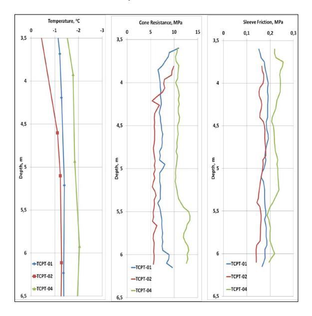
Figure 14: Temperature, Cone Resistance q<sub>c</sub> and Sleeve Friction f<sub>s</sub> vs Depth for EGE-03
