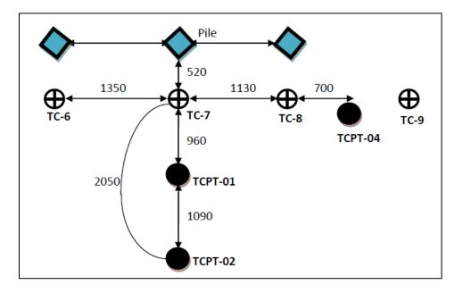
Figure 11: Location Scheme of Piles, Thermosyphons (TC) and TCPT Tests
