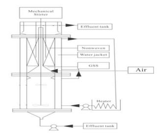
Figure 1: Schematic diagram of hybrid anammox reactor (HPNA).
