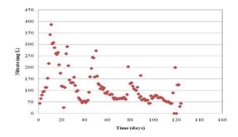
Figure 7: Time course of effluent nitrate concentrations in HPNA reactor
