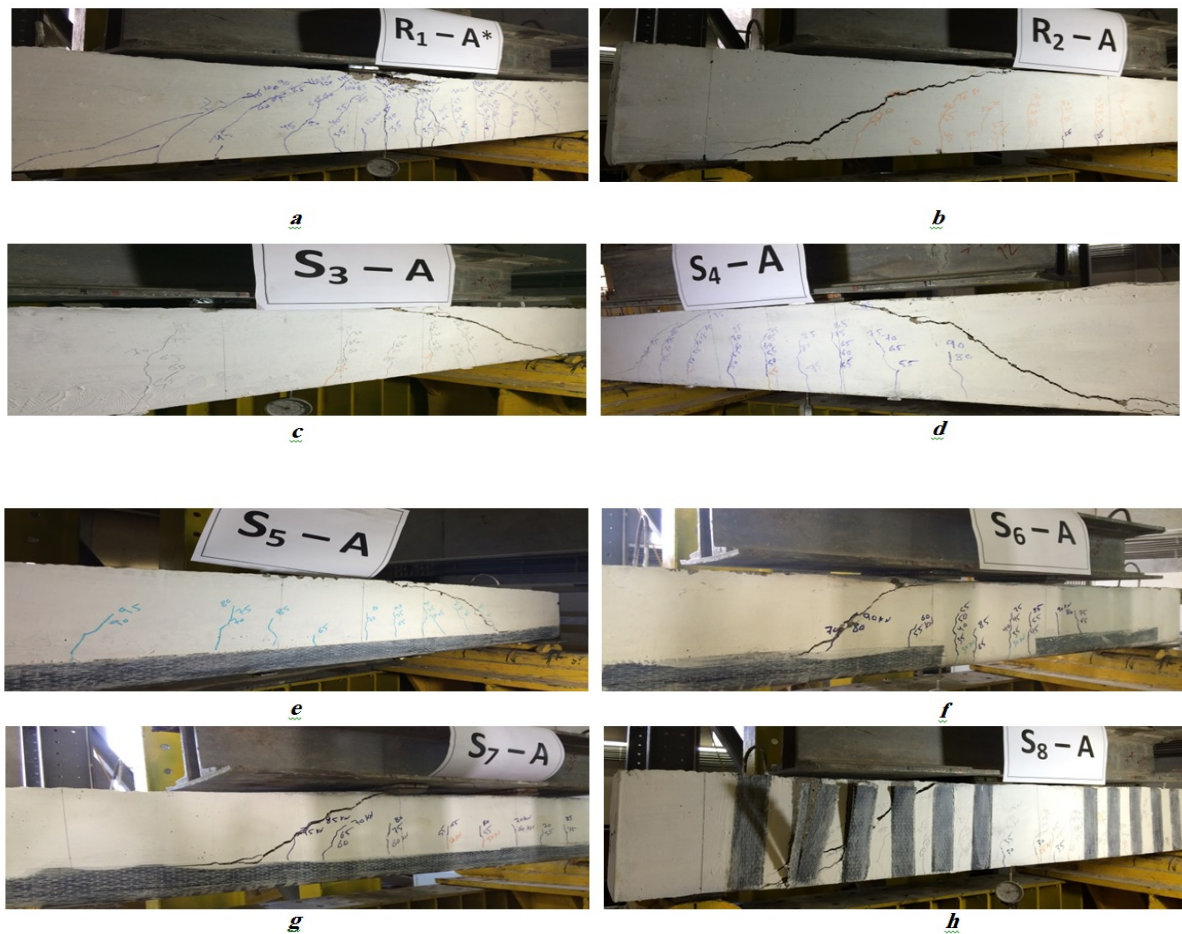
Figure 8: Typical failure modes for specimens Group A.
