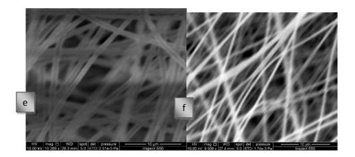
Figure 3: SEM images of pure and doped ZnO thin films: a-Pure ZnO, b- 1 % wt-Al, c- 2 % wt-Al, d- 3 % wt-Al, e- 4 % wt-Al, f- 5 % wt-Al
