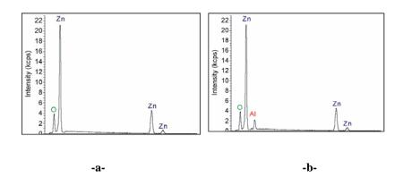
Figure 2: EDX analysis of pure and doped ZnO thin films: a- Pure ZnO (left), b- 5 % wt-Al (right),
