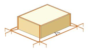
**Figure 4:** Type B earthing system with additional elements [6]
