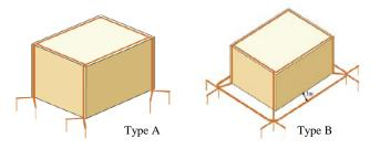
**Figure 1:** Type A& Type B earthing systems [4]
