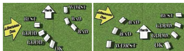
Figure 1: Best directions for buildings with least need for vertical screens to prevent overheating [10].
