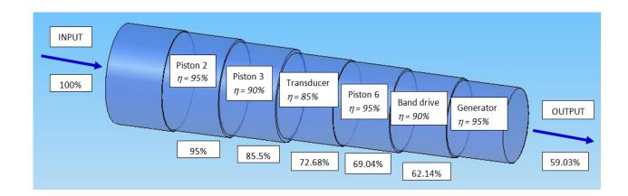
Figure 4: The average efficiency of device expected.
