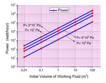
**Figure 5:** Power for 4 different values of pressure  $(10^6, 5 \cdot 10^6, 10^7 \text{ and } 2 \cdot 10^7 \text{ Pa})$ , and for 5 values of initial volume of working fluid (0.01, 0.1, 1.0, 10 and 100  $m^3$ ). The thermal expansion coefficient of working fluid is  $\beta = 1200 \cdot 10^{-6} \text{ K}^{-1}$ . Assumed that the temperature increased linearly for 10 °C during 10 hours.
