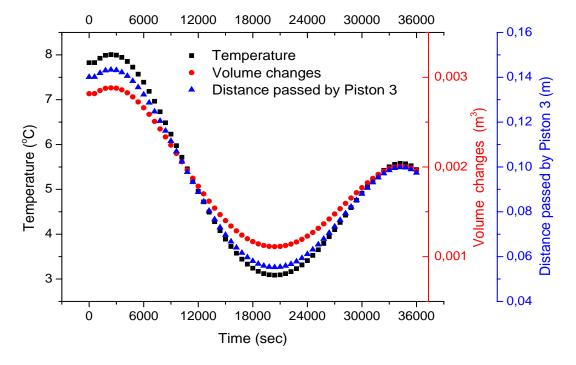
Figure 2: Changing of temperature, volume of working fluid and distance passed by Piston 3 with time.
