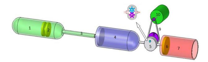
**Figure 1:** General principle scheme of the power unit. 1 – hydraulic preamplifier; 2, 3 and 6 – are pistons; 4 – main hydraulic amplifier; 5 – transducer; 7 – hydraulic cylinder; 8 and 9 – are band drive; 10 – generator.
