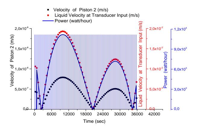
Figure 3: Velocity of piston 2, liquid velocity at transducer input and power during considered time.
