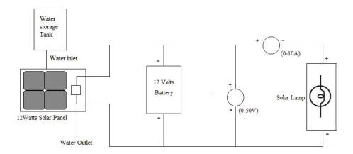
Figure 1: Output characteristics test system of solar panels with water cooling.
