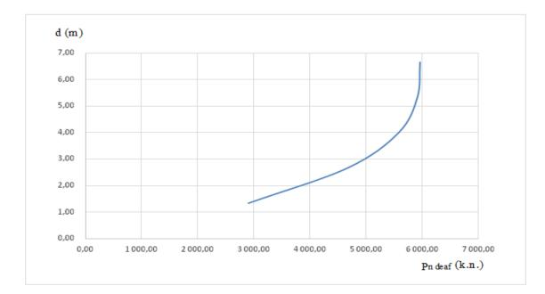
Figure 6: The functional defendence between changeable diameter of cylinder shape elements and residual attacking force of debris flow action on the deaf section of the construction after pass through type debris flow **against** construction
