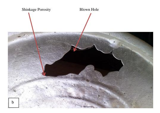
Figure 4 (a & b): Cast Components showing some Defects
