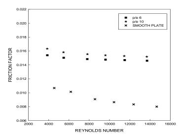
Figure 5: Effect of Reynolds on friction factor with variation relative roughness pitch as compare to smooth duct for W-discrete ribs flow arrangement.
