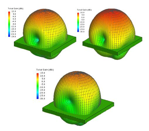
Figure 9: 3-D dimension results of gain produced by FEKO in x-y plane at different sizes of ground plane
