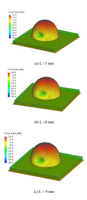
Figure 5: 3-D dimension results of gain produced by FEKO in x-y plane at resonant frequency (a): f = 12.57 GHz (b): f = 12.61 GHz (c): f = 12.62 GHz
