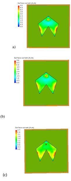
Figure 4: 3-D dimensionresults of current distribution produced by FEKO at f =12.5 GHz in x-y plane (a): L = 7 mm (b): L = 8 mm (c): L = 9 mm
