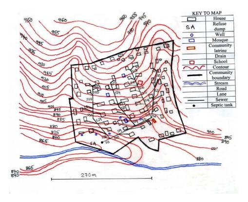
Figure 3: Topographical map of research community (Kotoko) showing proposed sewers connected to 42 households without sanitation facilities
