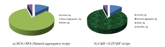
**Figure 1**: Reduction of using the generic material by using the recycled C&D waste in Tanzania (adopted from [14])
